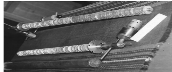
Figure 8. VDT (stainless-steel/water) with mini gas burner. Sorbent material in disposed between fins.
