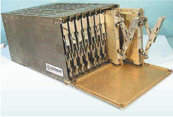
Figure 8. Rack and LRMs configuration
