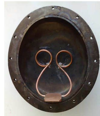
Figure 4. Top cap of the compressor with fitted PLT
