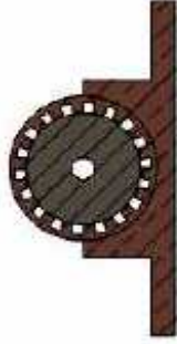
Figure 2. Cross section of the card LHP evaporator
