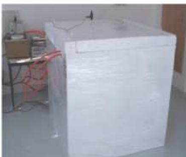
Figure 1. Thermostatic chamber for testing cooling by natural convection
