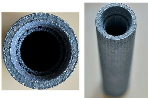
Figure 8: Arterial wick heat pipe made from AlSi12. (Small ducts inside the wick can be seen)
