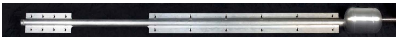
Figure 1. A typical VCHP with an evaporator, a single condenser, and an electrically heated reservoir at the end of the condenser.
