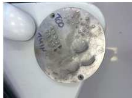
Figure 1: In SLM machine, objects are made on a substrate and then are cut using a wire erosion process. A substrate is shown here with some random geometry fabricated on it.
