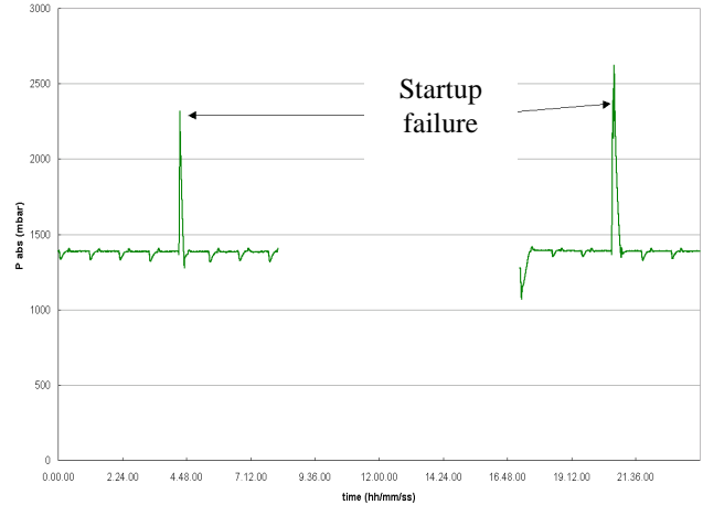
Figure 7. Pressure evolution during startup cycling at 1 kW (19 w/cm 2 ) : 2 failures for 14 startups.
