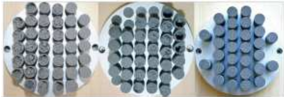
Figure 7: Porous samples made for permeability measurements. Different tries improved the quality as shown above from first build on the left to the 3rd build on the right
