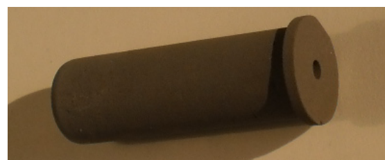
Figure 10. Machined porous wick (nickel)
