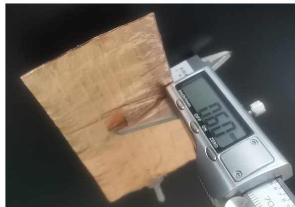
Figure 2. Ultra-thin flexible flat heat pipe
