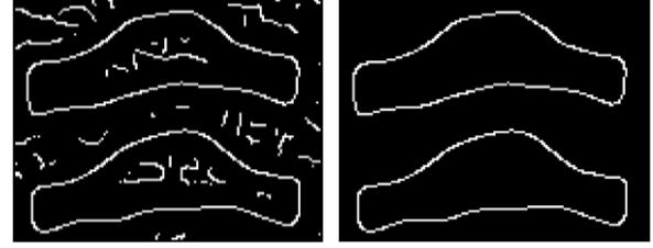
Figure 10. Canny edge detection example of Heat Exchanger channels with threshold value of 0 (Left) and 0.2 (Right).
