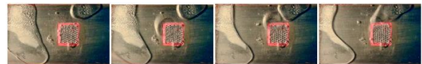
Figure 3. Formation and coalescence of bubbles on heated surface with pillars, v = 0.006 m/s, 60 W.
