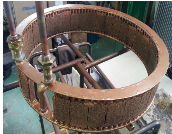
Figure 2. Evaporator with metal foam of loop type two-phase thermosyphon
