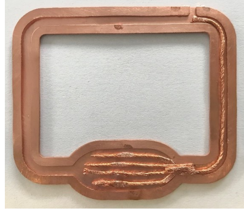
Figure 1. The novel porous media of twisted copper wires inside the LHP.
