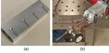
Figure 10. Heating System. (a) Heating block. (b) Heaters attached to the instrumented heat pipe.
