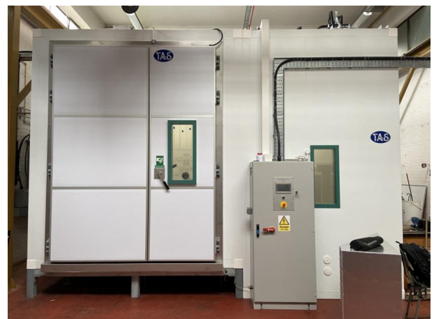
Figure 3. TAS Environmental Chamber at University of Brighton used for the tests presented in this work.
